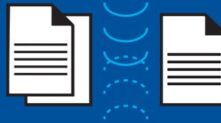
Multifeed detection uses sound waves to identify potential misfeeds, reducing the risk of damaged documents and lost data.
